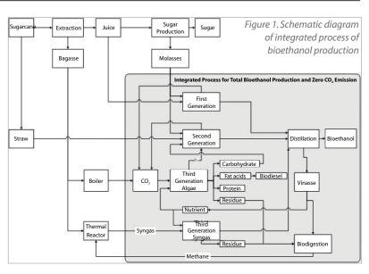
fermentation of synthesis gas. This challenging integrated process has the major appeal of not emitting carbon dioxide and makes the best of the carbon-containing material for producing ethanol, turning it, when technically and economically feasible, a milestone for improving Brazilian bioethanol competitiveness.
